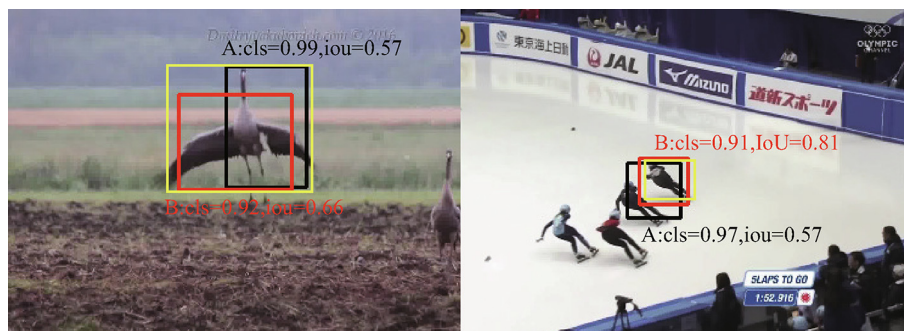
Fig. 2. Illustration for the problem of mismatch between the classification scores and bounding box estimates. The yellow boxes are the ground truth. The black estimated bounding boxes (denoted as A) have higher classification scores but lower IoU scores than the red bounding boxes (denoted as B). Best viewed in color.
